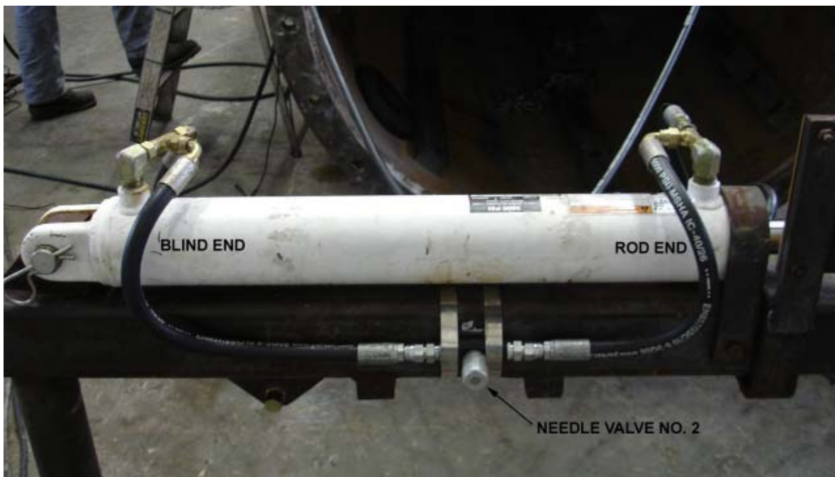
Figure 2-H. Visual Stroke Indicator Cylinder - Rear
