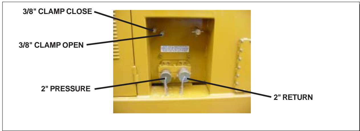
Figure 2-F. Power Unit Coupler Layout
