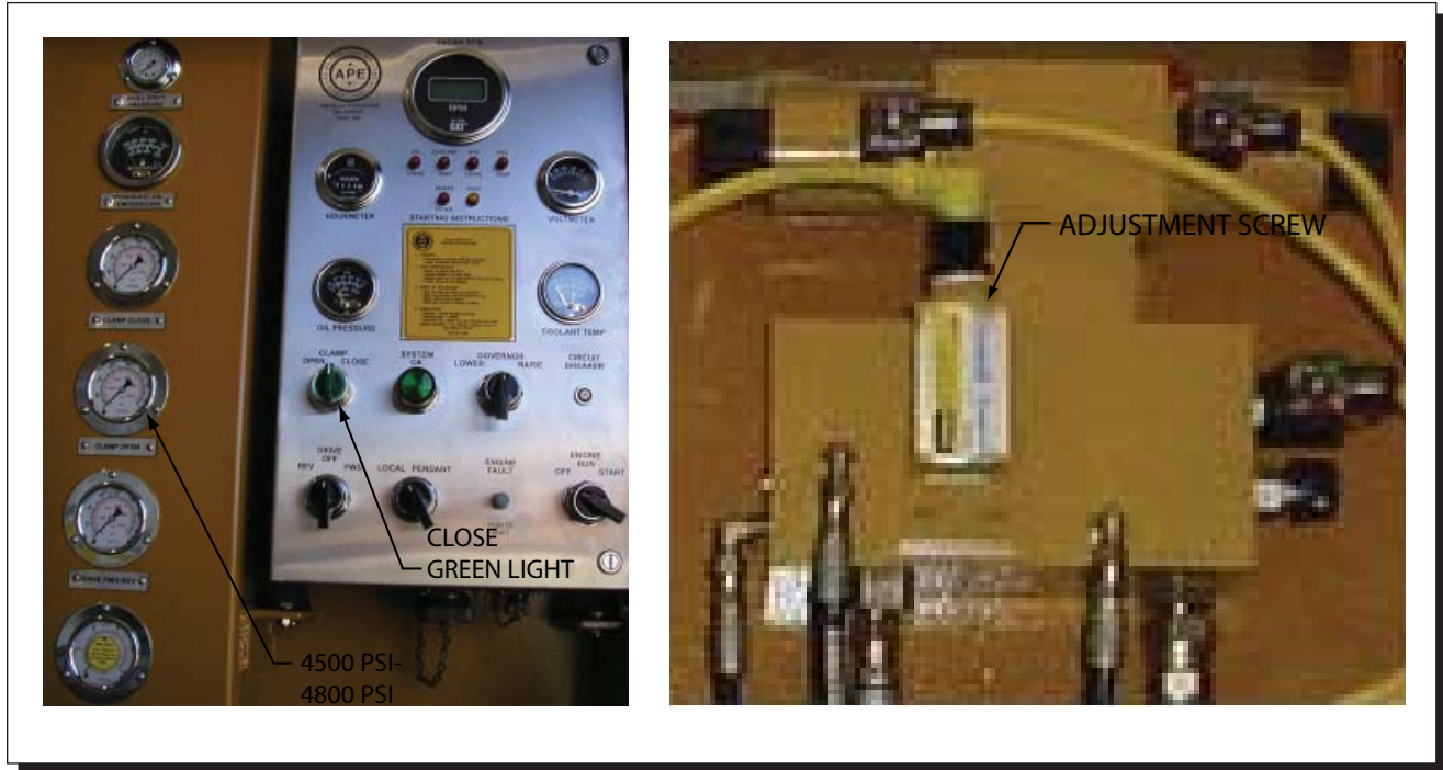
Figure 4-D. Checking Clamp Pressure Switch Setting
