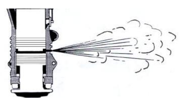
Note: Water can build up in the combustion chamber from rain or from condensation. If not removed, this water can be forced up the injector and into the fuel pump or even into the fuel tank. Water is the main source of downtime on a diesel hammer. Blow out your hammer each morning.
