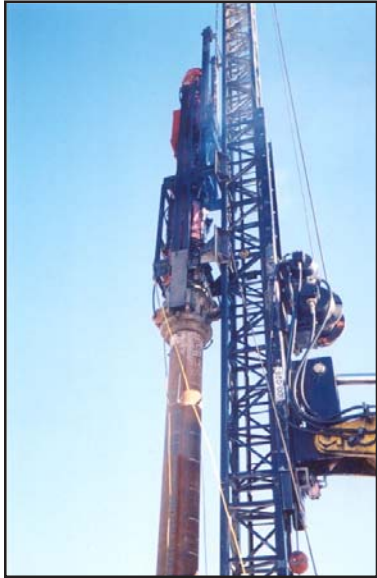
D25-42 with Excavator Mounted Leader.
